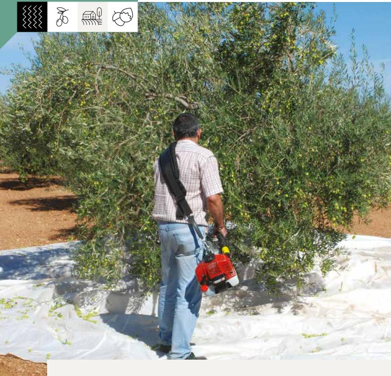
The **SC800** olive shaker is the professional olive harvesting machine. A group of users equipped with nets and SC800 olive shaker can harvest more than 15 quintals of olives per day with a 95% drop of the fruit, without damaging the tree or its cabbages. The anti-vibration system in the handles minimizes the vibrations transmitted to the user, who will appreciate the results obtained, the proven reliability and durability of the machine.
